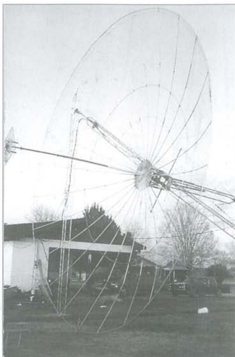
W5VUY 30ft hb dish with 3/4 & 1/2" electr. cond. + chicken w
